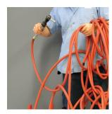
Hoses are often left lying on the workshop floor. This increases the risk of injury and equipment damage. Improperly stored hoses or kinked hoses lead to premature wear and the risk of hose puncture, which can cause dangerous hose whip.
